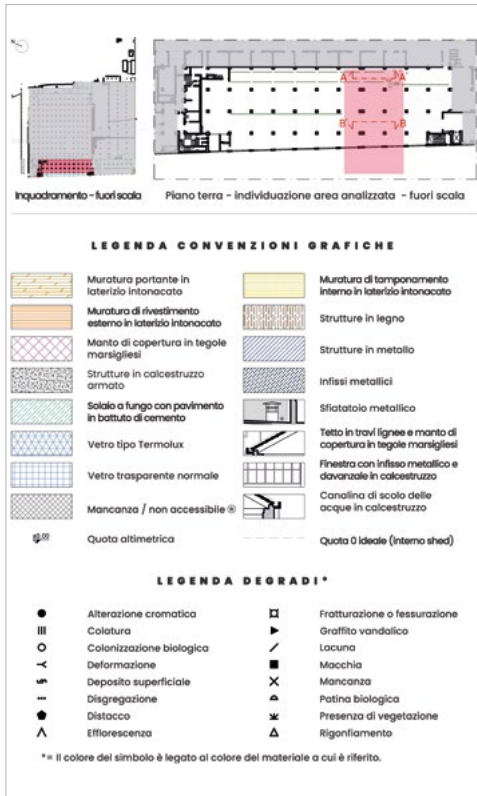
Fig. 8 - The former Pettinature Rivetti in Biella (BI), sections - interior elevation, material survey and analysis of the state of conservation (original drawings on a scale of 1:50, 2021).
