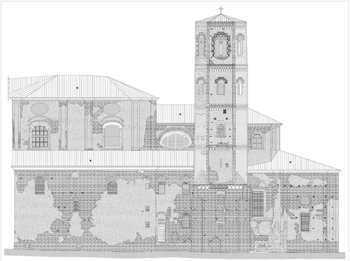
Fig. 2 – Detailed survey of the north front of the church of Santa Maria of Lucedio and the bell tower with the key of the graphic symbology (original drawing scale 1:50, 2006).
